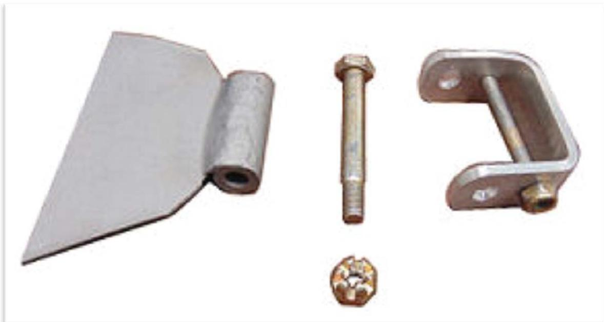
The pivot bolt (center) is an AN4-21 and the clamp bolt is an AN3-21.
