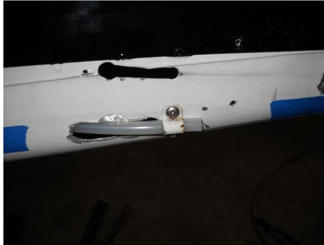
8. Cut two 1/8" 7x19 cables 166" long. Use masking tape over the cut to keep the cable from coming apart, and cut with a Dremel tool with a cut off wheel attached. Slip a piece of 1/4" heat-shrink tubing over the cable.
