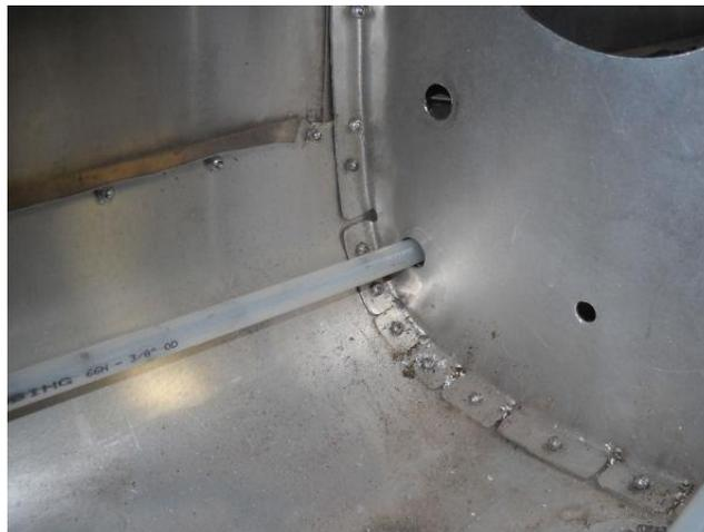
7. Using the old rear Teleflex cable clamp, secure the nylon tube as shown aft of F10.
