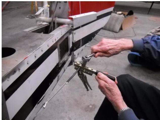
10. Attach the cable at the rudder pedal brake pivot bolt and thread it into the nylon tube until it comes out the rear.
