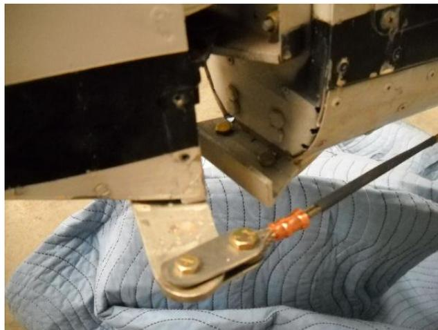
13. With the aft cable end assembled and clamped with vice grips, check for neutral rudder and neutral rudder pedals. Swage the sleeves three times each.
